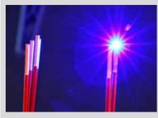
Laserline is optimising its portfolio in the LDMblue high-power diode laser segment with 450 nm wavelength. Primarily developed for copper material processing in the electronics industry, these blue diode lasers are now available in six power levels between 300 and 2,000 watts.
