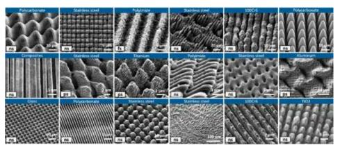
Figure 1: Different microarchitecture designs realised using Direct Laser Interference Patterning.
