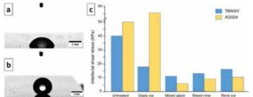
Figure 2: (a) Exemplification of the change in water contact angle on the reference (top) and DLIP-treated surface (bottom) for Ti6Al4V. (b) Ice adhesion of the laser-textured surfaces as measured by the interfacial shear stress under different atmospheric conditions for Ti6Al4V and Al2024 alloys.
