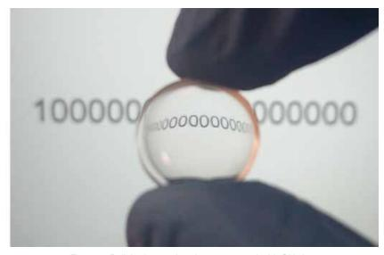
Figure 5: Polished curved surface processed with GHz burst.
