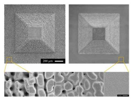
Figure 2: SEM collage of structures fabricated in stainless steel. From 6 µm to 200 nm Sa surface roughness achieved. Results demonstrated by Fachgruppe Physik und Lasertechnik, Laserinstitut Hochschule Mittweida.
