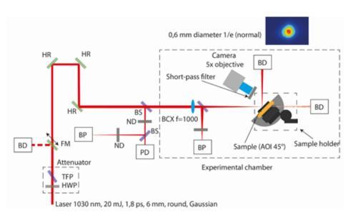
Figure 1: LIDT station layout designed at HiLASE (for Perla laser). HWP - half wave plate, TFP – thin film polariser, FM – flip mirror, BD – beam dump, HR – highly reflective mirror, BS – beam sampler, ND – neutral density filter, PD – photodiode, BP – beamprofiler.
