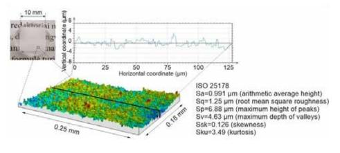
Figure 3: Hydrophylic acrylic polymer surface roughness after ablating using MHz
