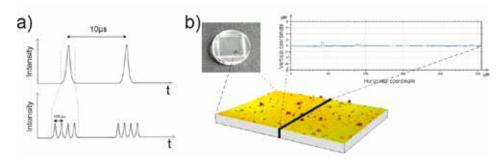
Figure 4: (a) Femtosecond laser pulse divided into bursts, (b) hydrophylic acrilic polymer after polishing parameters used: avg. power = 30 W, scanning velocity = 1 m/s, scanning pitch = 10  $\mu$ m, number of GHz pulses = 10
