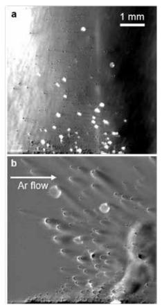
Figure 1: Schlieren images of LPBF (a) without cross-flow (b) with cross-flow. Videos for all images available with [3].
