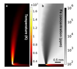
Figure 4: Calculated (a) temperature and (b) Fe content over the melt pool.
