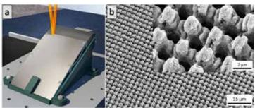
Figure 3: (a) Representation of the 3D processing of the NACA profile through DLIP and (b) resulting microstructures on the Ti6Al4V airfoil.
