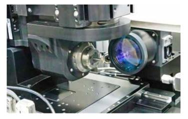
robot was integrated along with other additional components such as an optical measuring system for in-process measurement. The advantage here was that the same Aerotech control system could be used. "This allows us to expand the periphery at any time without having to purchase new control software, for example if we want to integrate a Profibus or an additional piezo axis - we are absolutely open and not restricted at all."
