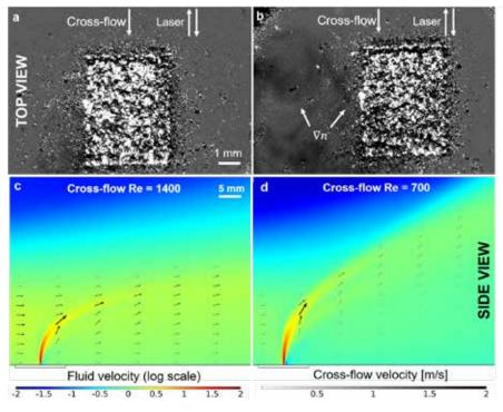
Figure 3: High (left) and low flow (right) comparison. (a - b) Direct imaging during layer 30, showing higher atmospheric fume content under low flow. (c - d) Velocity plot, suggesting plume is not incorporated in cross-flow stream under low flow.
