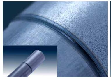
Laser welding of medical cannisters for device encapsulation e.g. implantable defibrillator battery cans.
