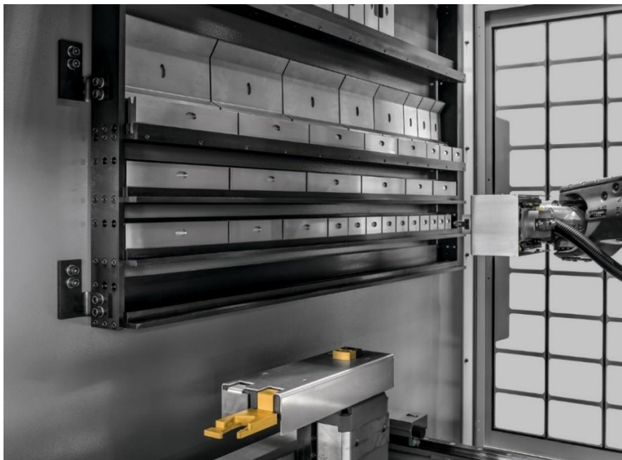
Shorter setup times thanks to the Modular Tool Changer.
